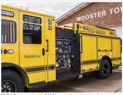
IDEX Corporation's SAM control system assists pump operators in managing waterflow, so their focus is on the fireground and the attack crew – not the fire truck.
