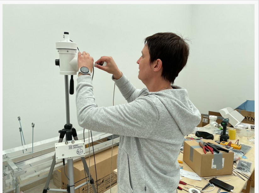
Prof Kathy Steppe - Universiteit Gent - fitting Vaisala GMP252 CO 2 probe to weather station
