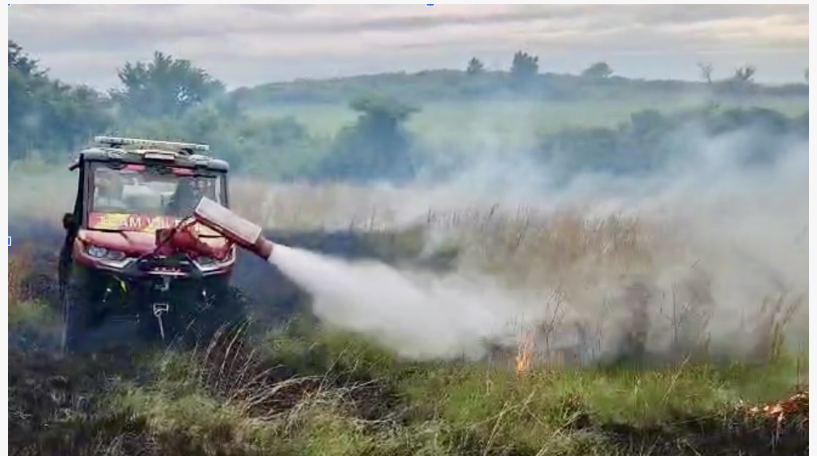
Team Wildfire's Storm Cell demonstrates its ability to rapidly and efficiently suppress wildfires with proprietary jet engine technology.
