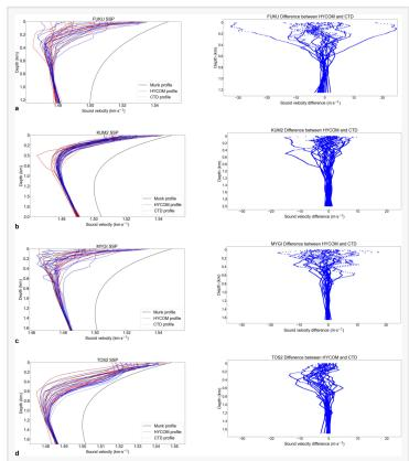
Comparison of the in situ profile, HYCOM profile, and Munk profile sound speed at the four sites FUKU a, KUM2 b, MYGI c, and TOS2 d.
