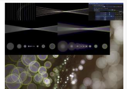
Bubble bokeh from over-corrected spherical aberration
