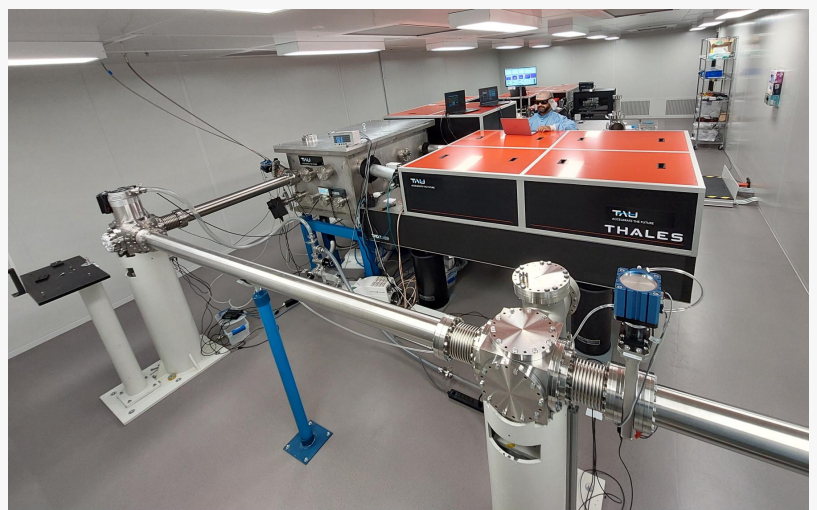
TAU Systems' particle accelerator, driven by Thales' laser
