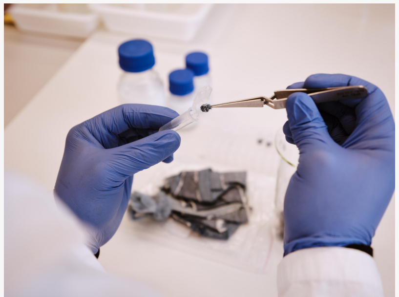
Confirming material authenticity: DNA is extracted from denim to prove it's truly recycled.
