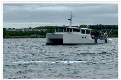
Raytheon and CET's extended-range uncrewed undersea vehicle (UUV) surfaces in Narragansett Bay following a successful autonomous in-water demonstration in just four months after initial concept.
