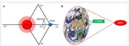
The schematic diagram of the DSCOVR satellite in the Sun–Earth space (A), and the EPIC and CERES for Earth observation (B), in which the background image was captured by DSCOVR/EPIC at 00:17 on 2024 May 1. The distances are not to scale.
