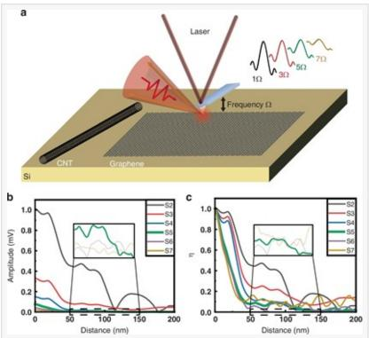
Schematic of s-SNOM principle and comparison of higher-order signals (2nd–7th). a The schematic diagram of the measurement principle of s-SNOM. b The electric field strength from the 2nd to the 7th order. c Signal-to-noise ratio (SNR) values from the 2nd
