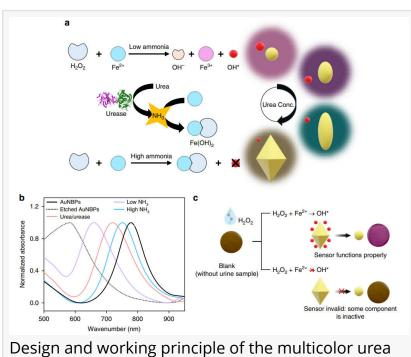
Design and working principle of the multicolor urea biosensor.
