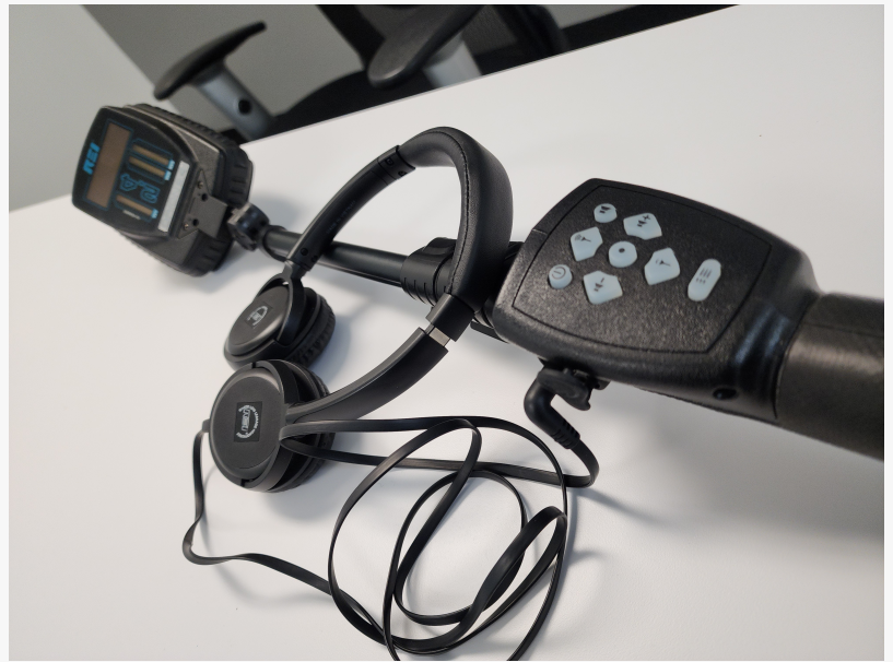
A Non Linear Junction Detector is one of the essential TSCM tools used.
