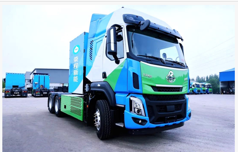
Rockcheck Heavy Duty Truck Powered by 400kW Horizon Fuel Cell
