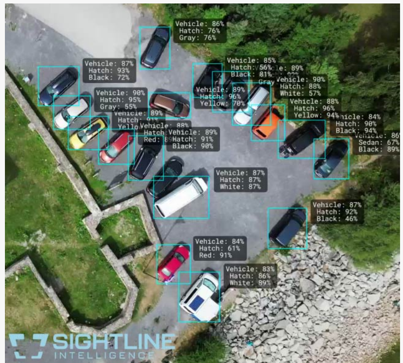
Sightline Intelligence AiTR Multi-Stage Classifier for Vehicle-Type-Color
