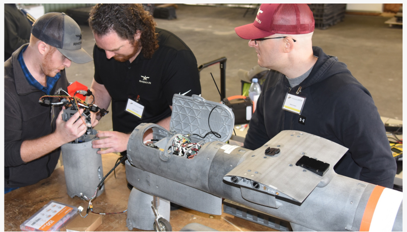
Rhoman Aerospace integrate their GPS-denied autonomous navigation and maneuvering system into Firestorm Labs' modular Tempest drone during a Naval Postgraduate School JIFX event.
