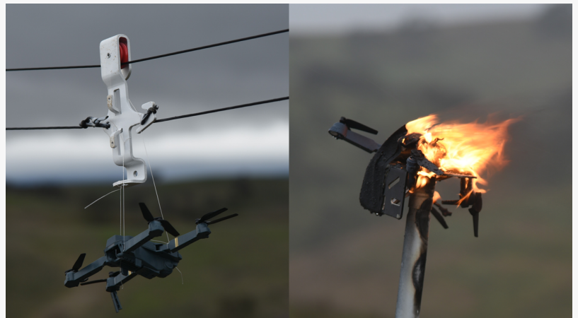
Aurelius Systems tested its laser weapon system (LWS) at Naval Postgraduate School's JIFX. Firing at static and towed quadcopters, the LWS recognized the drones as targets.
