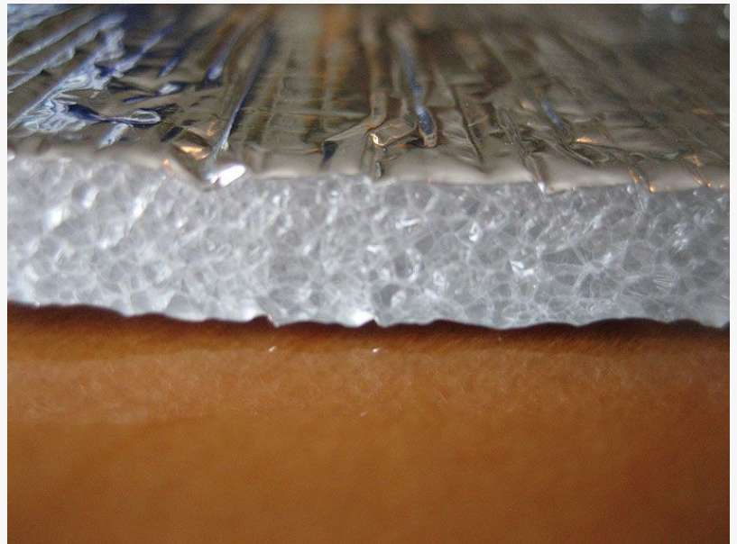
Closed cell foam of Prodex Total Insulation
