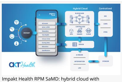
Impakt Health RPM SaMD: hybrid cloud with blockchain integrity and EHR/EDC/CDMS/RTMS connectivity for care & research.
