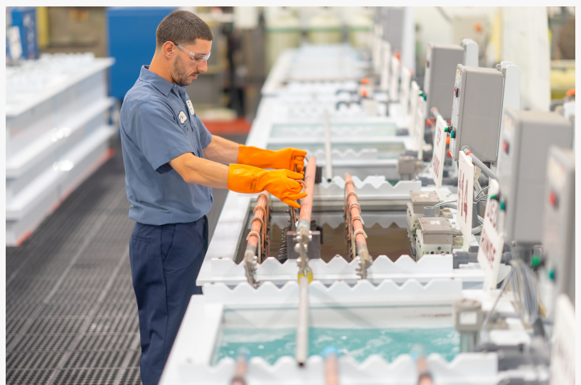
Electropolisher electropolishing stainless steel components
