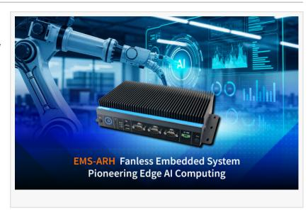
EMS-ARH modular fanless embedded system. Powered by Intel® Arrow Lake-H Core™ Ultra 7/5 processors and featuring integrated Intel® Arc™ GPU and NPU AI engines, EMS-ARH delivers up to 99 TOPS of total AI performance — providing a robust and scalable platform for diverse edge AI applications.
