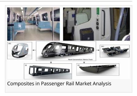
are gaining traction due to their remarkable strength-to-weight ratio and durability. These materials are revolutionizing the manufacturing of various components within passenger trains, offering benefits such as weight reduction, enhanced fuel efficiency, and improved structural integrity. The use of composites in the passenger rail sector not only addresses the need for lightweight solutions but also contributes to a more sustainable and environmentally friendly mode of transportation.
