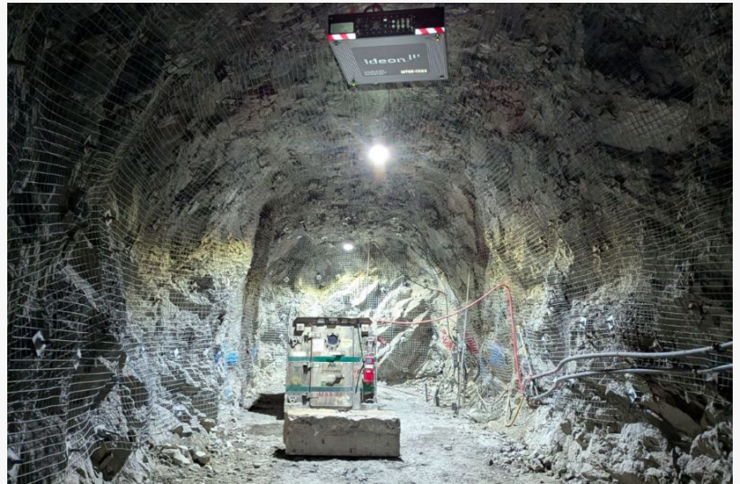
Ideon panel muon detector installed in-mine at the Pumpkin Hollow underground copper mine.
