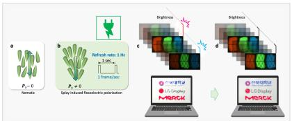
Fig 1. Schematic representation of molecular orientation and the low-frequency power-saving mode in fringe-field switching liquid crystal displays (FFS-LCDs). (a) Molecular alignment in the nematic phase. (b) Flexoelectric polarization induced at low flow frequencies.
