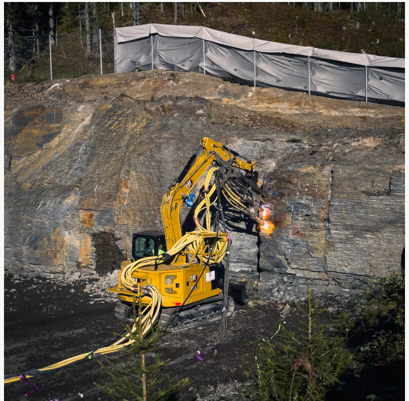
EarthGrid PBC's PES (Plasma Excavation System) conducting field testing near Trondheim, Norway
