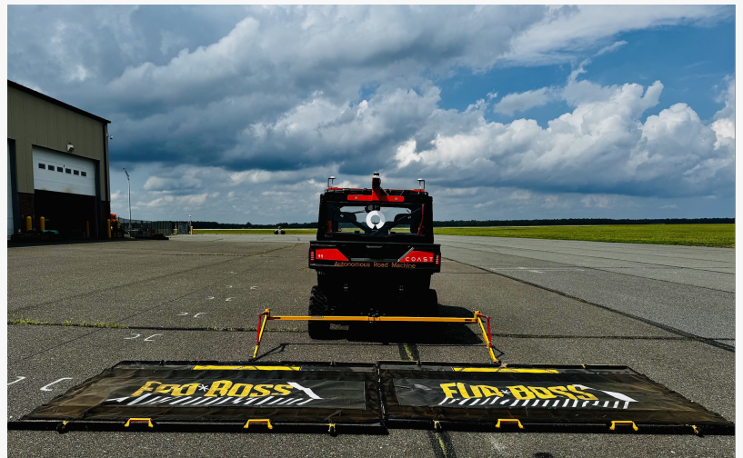
COAST Autonomous ProXD towing dual FOD*BOSS sweepers at Atlantic City International Airport, demonstrating next-generation automated runway debris removal technology
