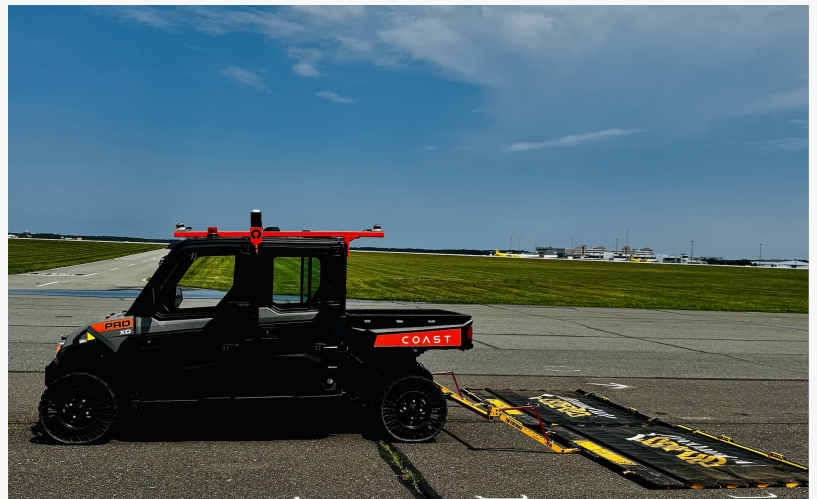
COAST Autonomous ProXD equipped with Aerosweep's FOD*BOSS on at ACY demonstrating advanced autonomous debris management technology in action for airport runway safety.
