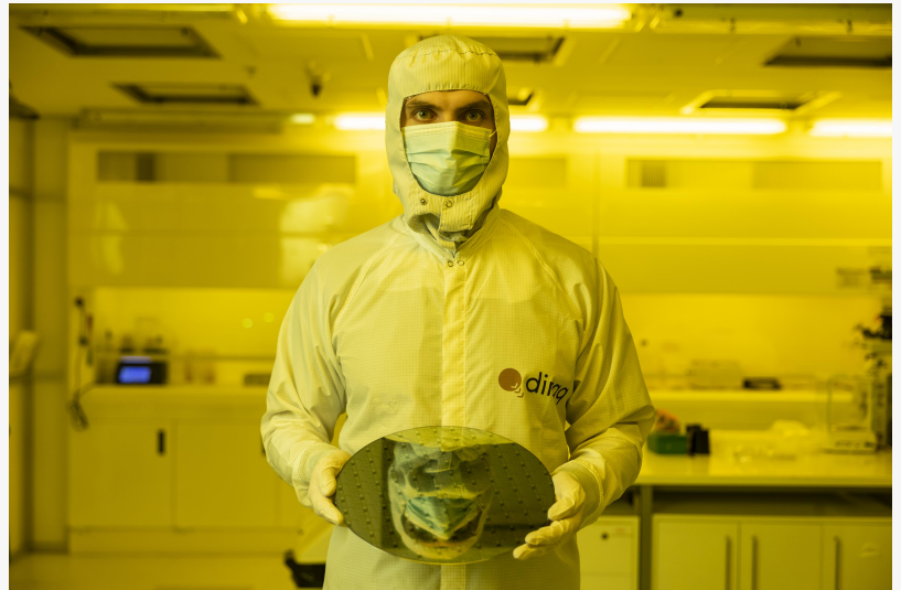
Diraq Measurement Engineer and lead author, Paul Steinacker, holding a 300 mm silicon wafer containing Diraq's quantum computer chips, which were manufactured at Interuniversity Microelectronics Centre (imec) using standard semiconductor processes.
