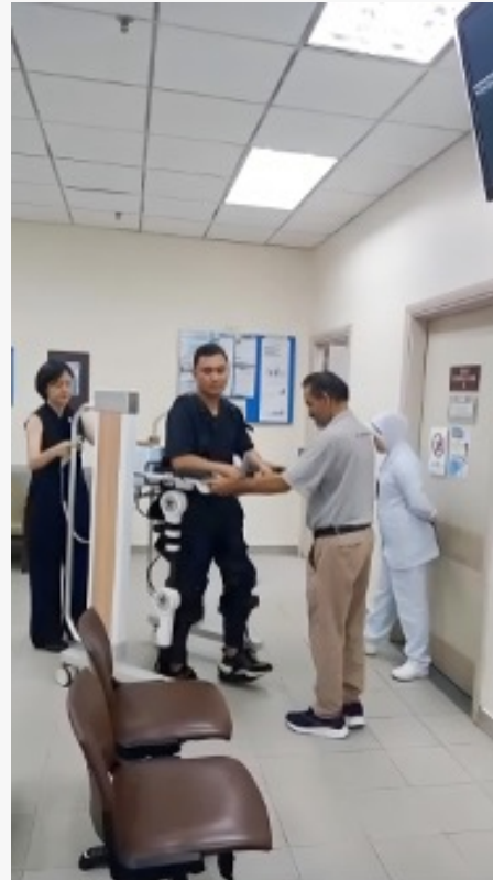
Clinician trial at HSB: therapist dons the UGO exoskeleton, testing fit, safety checks, and control interface before patient use.
