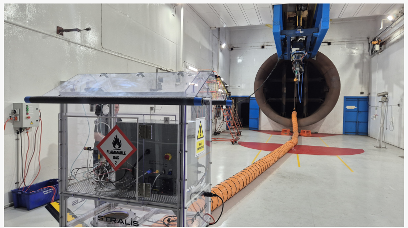
Stralis fuel cell test rig in the Air New Zealand's Engine Test Cell facility at Auckland Airport
