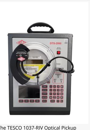
The TESCO 1037-RIV Optical Pickup Mounted on a TESCO Desktop Meter Station DTS-2990
