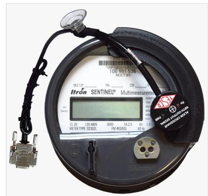
TESCO 1037-RIV Optical Pickup Mounted to an Itron Sentinel Meter
