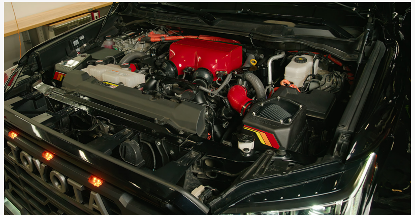
Engine bay view of Toyota Tundra with Magnuson Performance Pack.
