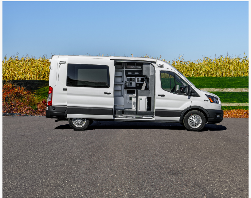
An FR Conversions Type II ambulance built on a Ford Transit ® 350 mid-roof chassis.
