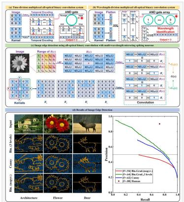
Fig.3 Demonstration of image edge detection based on microring resonators. (a) Time-division multiplexed all-optical binary convolution architecture; (b) Wavelength-division multiplexed all-optical binary convolution architecture; (c) Principle of image edge detection.
