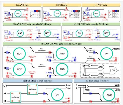
Fig 2. Illustration of all-optical digital logic gates using microring resonators. (a) AND gate; (b) OR gate; (c) NOT gate; (d) NAND gate; (e) NOR gate; (f) XOR gate; (g)-(h) Full adder.
