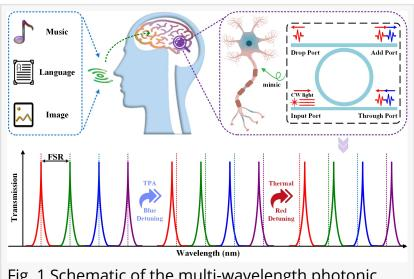
Fig. 1 Schematic of the multi-wavelength photonic spiking neuron based on microring resonators.
