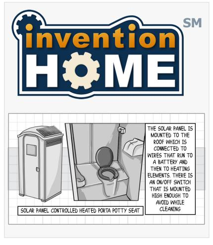
Users can activate the heating mechanism through a weather-resistant on/off switch positioned for accessibility while minimizing interference with cleaning or maintenance. This design is ideal for construction sites, campgrounds, hunting clubs, outdoor events, and other locations where portable sanitation units are deployed in cold climates. The Heated Porta-Potty Seat ensures that users can remain comfortable and benefit from offering a higher standard of service.
