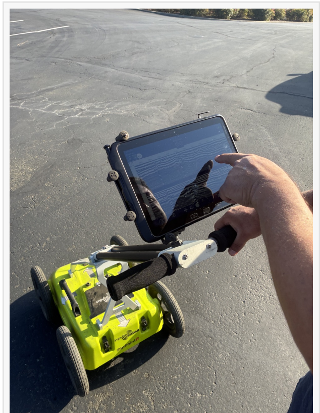
Showing proper way to read a Ground Penetrating Radar(GPR)
