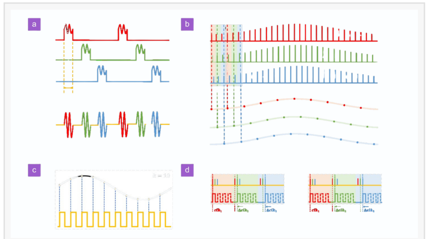
Fig. 2: (a) and (c) Schematic diagram and ADC clock phase of the conventional sampling method; (b) and (d) Schematic diagram and ADC clock phase of the proposed PMS algorithm.
