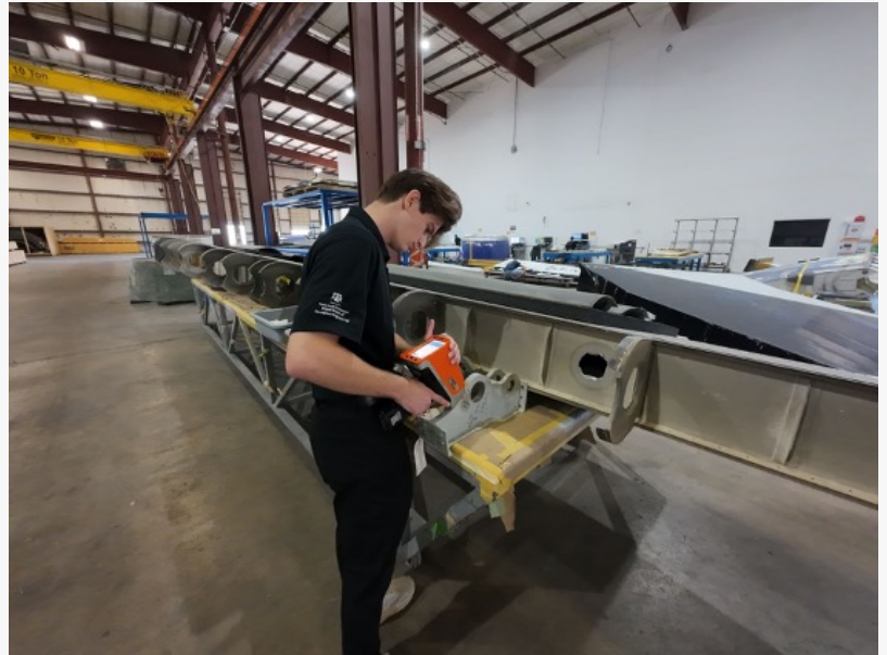
An ACD Consulting embedded engineer performing Non-destructive testing
