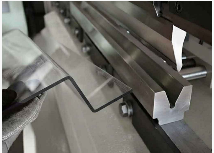
Clear polycarbonate sheet being bent on a press brake.
