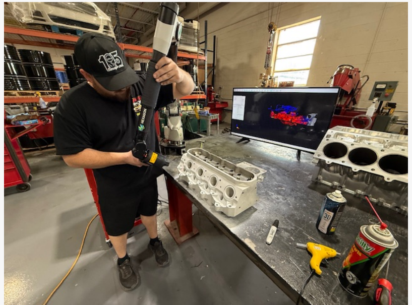
Shop Floor Fusion 360 scan of engine port
