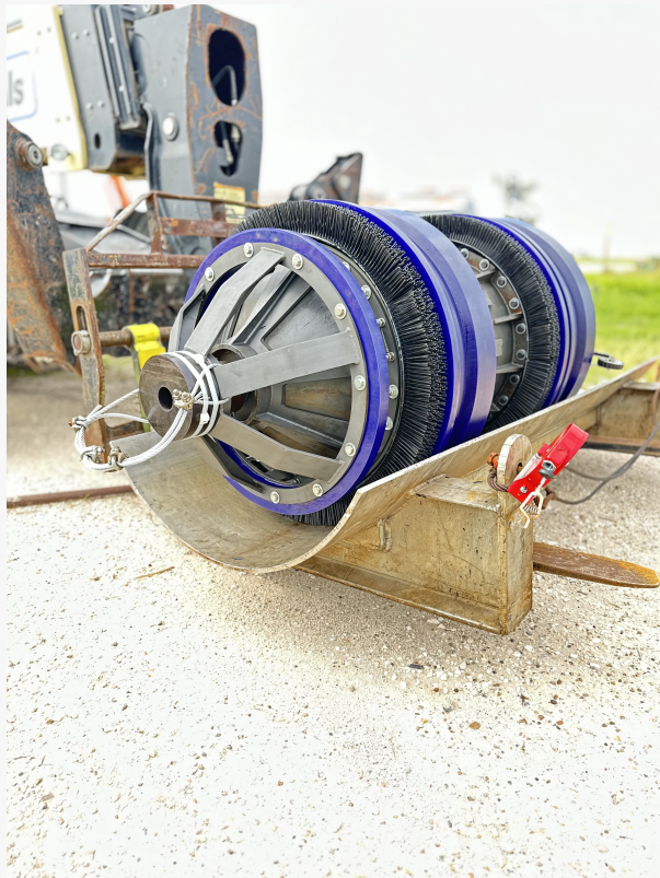
INLINE Services Speed Control Pig in Tray
