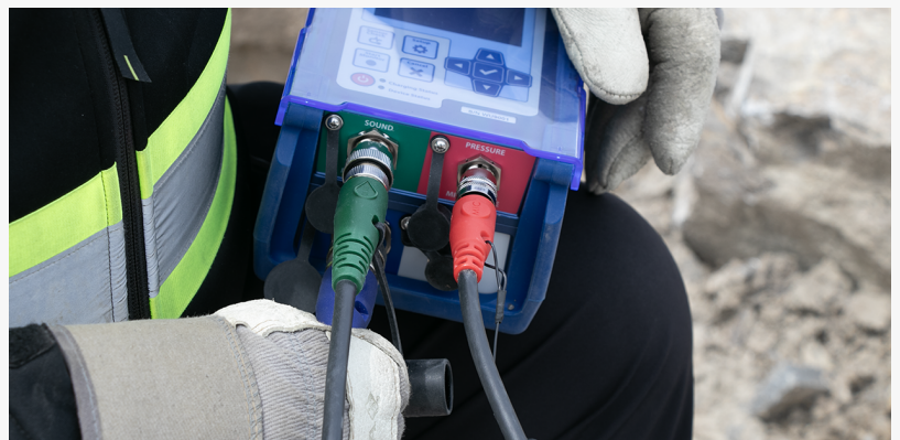
Monitor vibration, noise, and air overpressure simultaneously, all time-synchronized.
