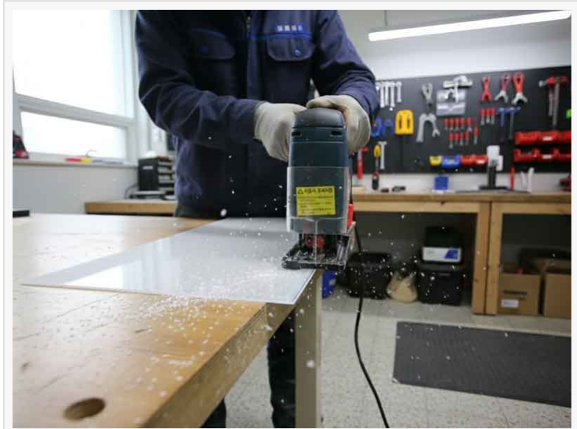
Acrylic sheet being cut with a jig saw.
