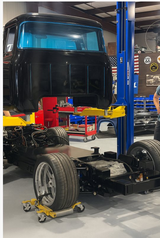
M100 body being mounted to the EV chassis
