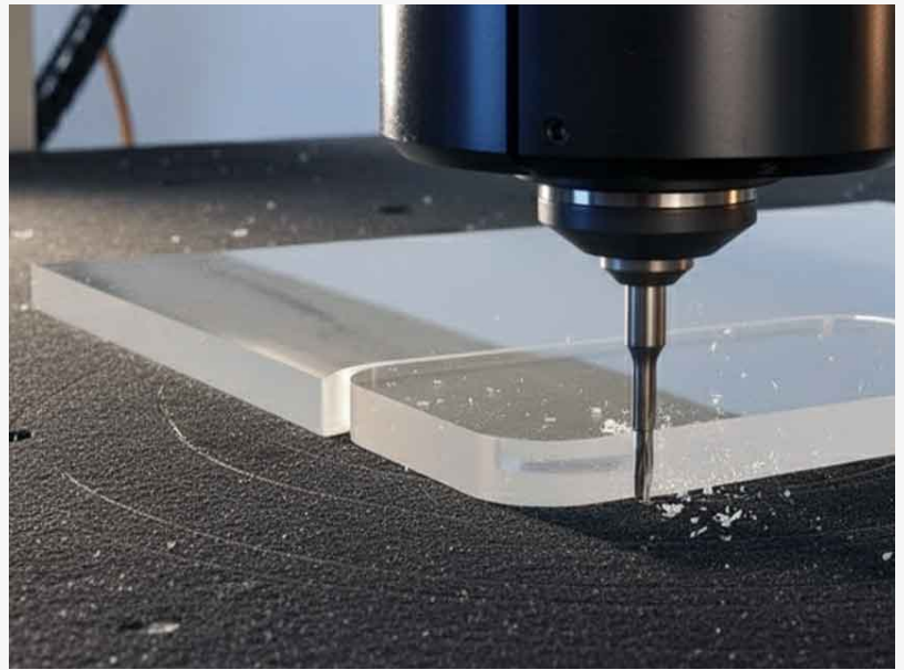
CNC router cutting an acrylic sheet, producing clean edges.
