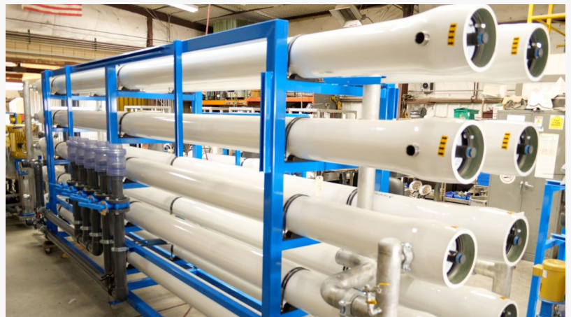
Progressive Water Treatment Reverse Osmosis Filtration System in Production
