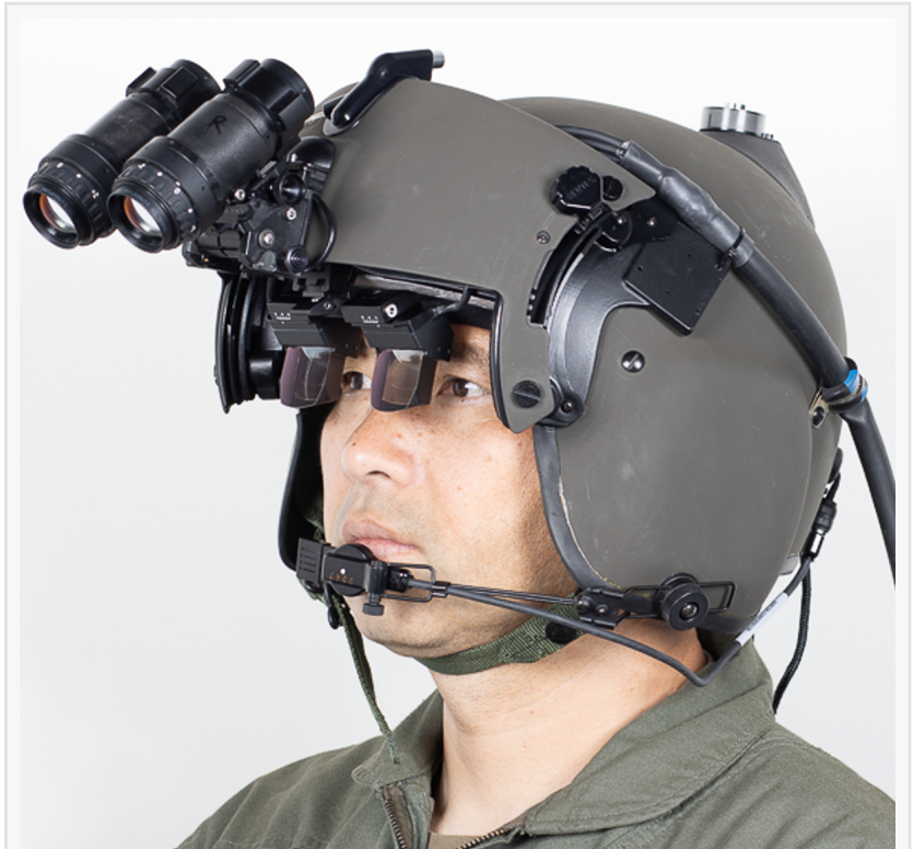
Vision Products' A3RO HMD for mitigating degraded visual environments
