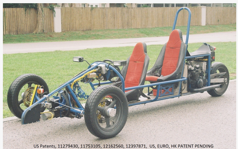
Three wheel motor vehicle. Two wheels in front, Drives like a car and Leans like a sport bike
