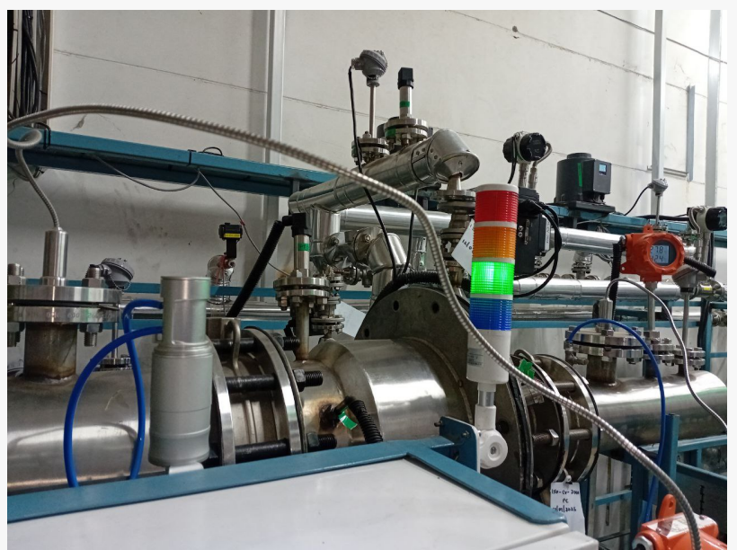
Vaisala GMP343 measures ppm level CO 2 at the inlet and outlet of the DAC plant with high accuracy and precision
