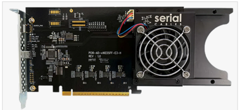
Hermes PCIe Gen6 x16 EDSFF-to-AIC Redriver Card supporting E1.S, E2, and E3.S/L SSDs for PCIe Gen6 validation.
