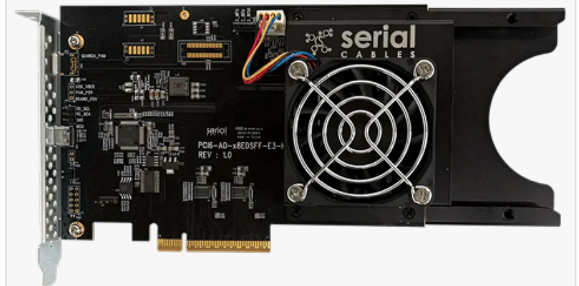
Hermes PCIe Gen6 x8 EDSFF-to-AIC Redriver Card supporting E1.S, E2, and E3.S/L SSDs for PCIe Gen6 validation.
