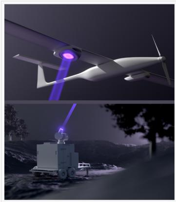
PowerLight is creating a "wireless power line" through the air, delivering kilowatt-class power over kilometers.
