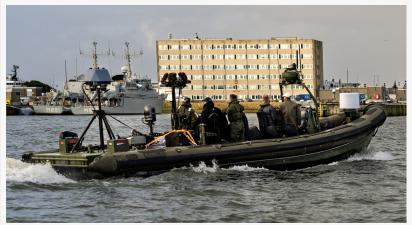
Aboard a Dutch Navy SOF fast raiding, interception, and special forces craft (FRISC) during the BOMA exercise, the Naval Postgraduate School c-UAS team deployed multiple sensors mounted to masts for detecting and identifying drone threats.
