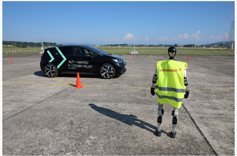
Testing Vehicle for obstacle detection and avoidance
